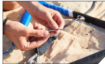
Wind the Trimmer Bracket screw back in.
