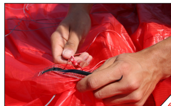
4 Disconnect the ISL line from the internal knot and pull the line out of the pocket. Ensure there are no tangles or knots in the line.
