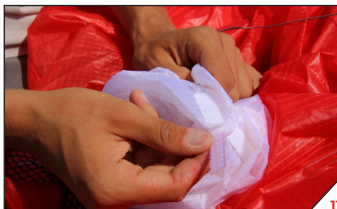
11 Reach inside the valve and attach the ends of the valve sock to the velcro retainer on the rib left and right sides.
