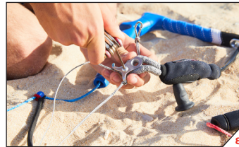
Wind the Trimmer Bracket screw back in.
