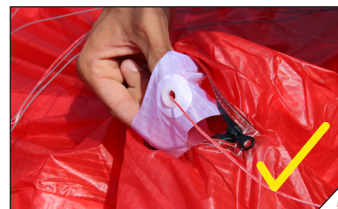
5 Ensure the ISL is not twisted around the Diagonal Rib inside.
