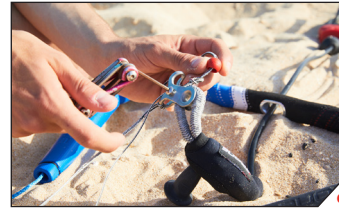
Remove the Trimmer Bracket screw.
