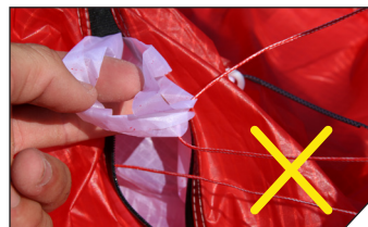
The line should be running freely from the neighboring rib to the zip opening.
