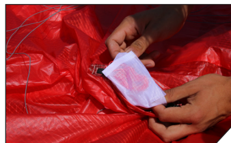
4 Disconnect the ISL line from the internal knot and pull the line out of the pocket. Ensure there are no tangles or knots in the line.
