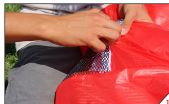
12 Close the Leading Edge air intake velcro.
