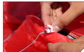
6 Feed the ISL line through the plastic ring on the bridle line tab next to the zip. Feed the line from the wing tip side towards the center.
