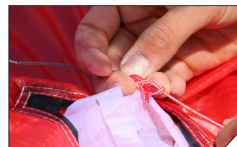
5 Connect the ISL line end to the internal knot using a larks head connection.
