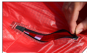
7 Close the zip until 5mm before the slider goes into the bungee cover, leaving room for the ISL line to run freely.
