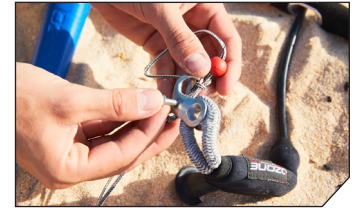
Pull line no.5 out through the Quick Release and bar centre.
