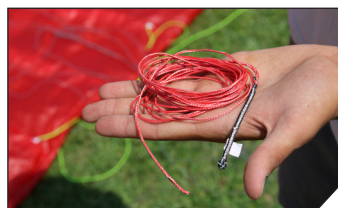
2 Unwind the LSL line. Ensure there are no tangles or knots in the line.
