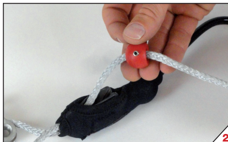
Pull the stopper ball and black webbing handle over the line.
