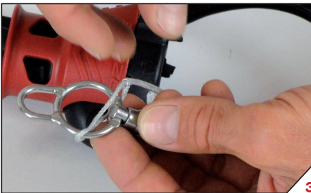
Put the stainless steel ring with swivel through the loop of the thin line and pull the bungy leader line all the way through.
